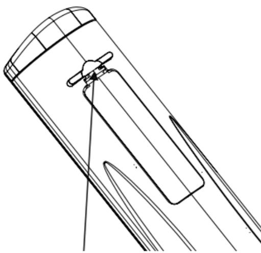
PRESS IN AND LIFT TAB TO REMOVE BATTERY COVER OUT FROM RECESS
