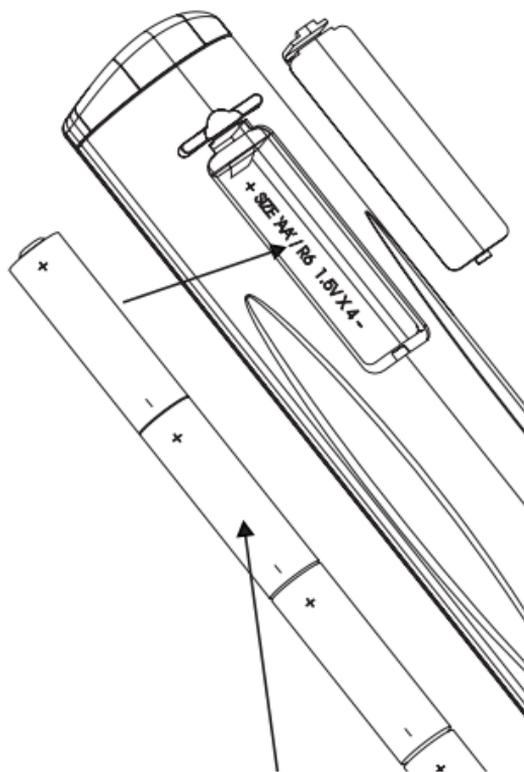
PLACE BATTERIES INTO OPENING. ENSURE THE CORRECT POLARITY IS OBSERVED
